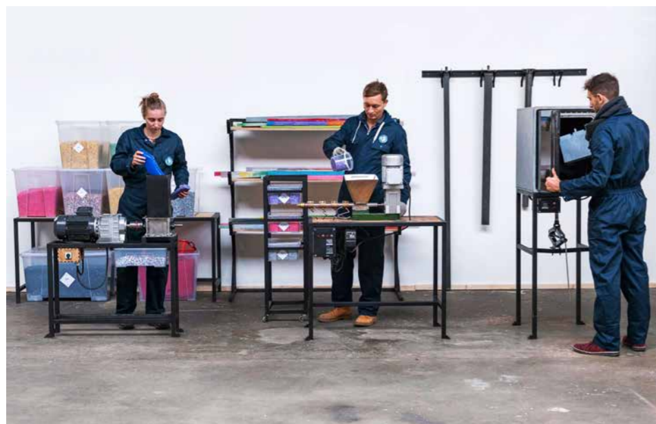
LEFT: Precious Plastic, machines for shredding, extruding and pressing plastic
