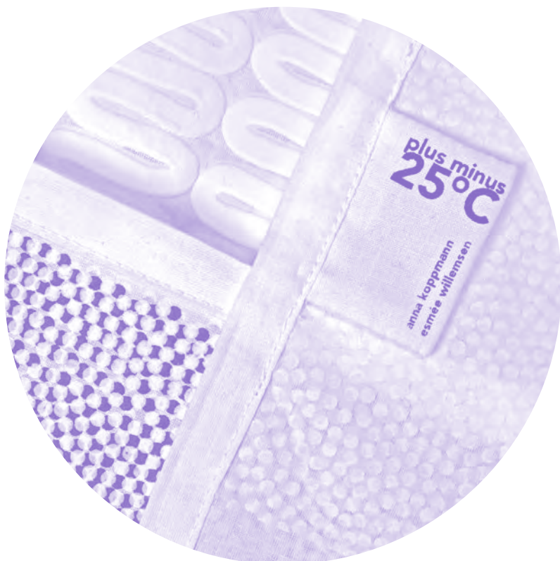
80 Plus Minus 25°C, curtain printed with phase-change material (PCM), by Anna Koppmann and Esmée Willemsen, 2020
